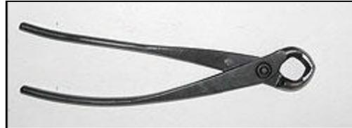
**Concave cutter:** *designed to cut branches and trunk, leaving a small indentation in the wood. The wound it leaves behind will heal with less visible scars. Essential.*
