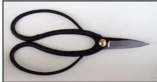
**Knob cutter:** *designed for removing branch stubs from trunks and branches, as well as for removing roots. Can also be used as a root cutter. Do not use in the soil and branch areas simultaneously. Essential.*
