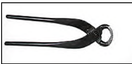
Root cutter: built strong enough for even the largest and oldest roots, they are essential if you plan on transplanting larger and/or older bonsai. They can also be used as a knob cutter. Not essential.
