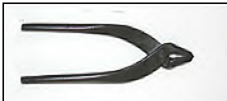
Straight pliers: helpful when wiring, removing branches, roots, and knobs from the trunk. Interchangeable with angled pliers. Not essential.
