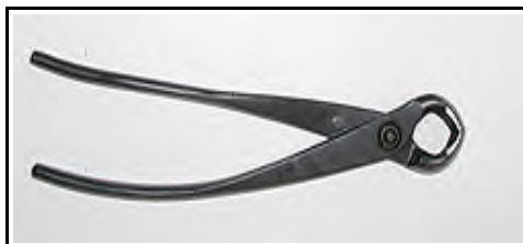
Knob cutter: designed for removing branch stubs from trunks and branches, and also removing large roots. Do not use in soil and branch areas simultaneously. Essential.
