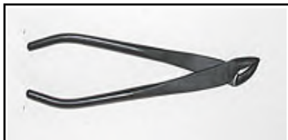
Angled pliers: used to crush branches strip bark and wood, creating dead wood (jin) and driftwood (shari). Not essential.
