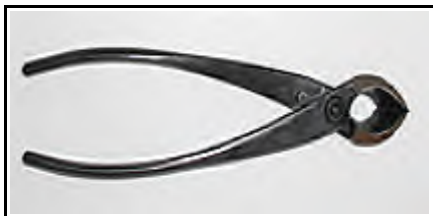
Concave cutter: designed to cut branches and trunk, leaving a small indentation in the wood, and thus less noticeable scars. Essential.
