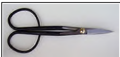
Twig shear: long narrow body, great for trimming buds and reaching deep without disturbing foliage. Not for general pruning as the blades will become dull sooner. Not essential.
