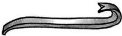
Illustration 1: A small wrecking bar or root hook are indispensable when working to examine the roots
